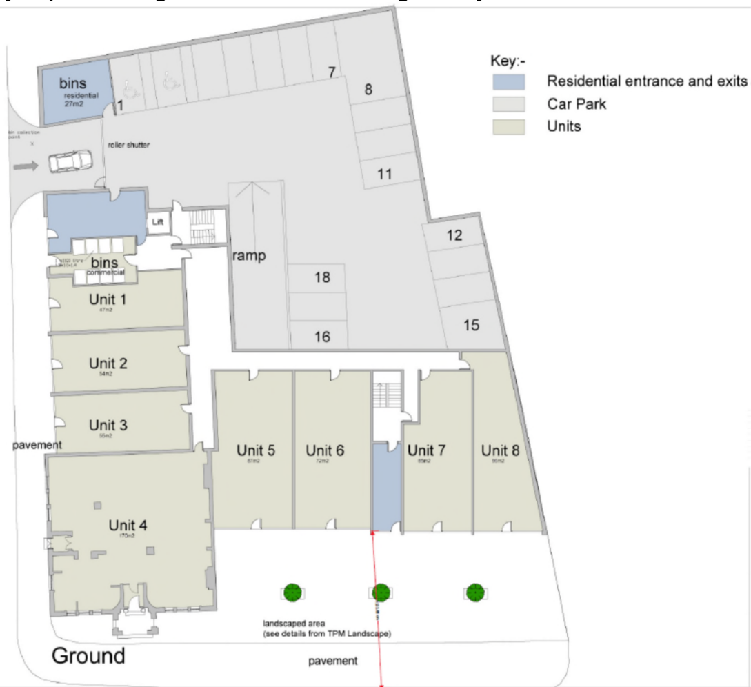
Proposed ground floor layout plan
